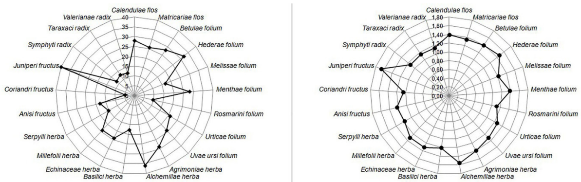
Figure 2. Comparison of compressibility index and Hausner ratio values for herbal drugs
