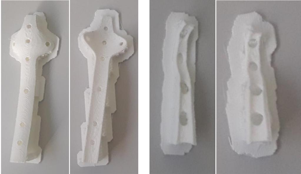
**Figure 41** .Plate models created by 3D printing.
