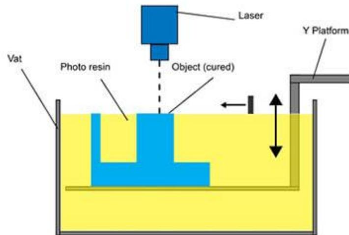
**Figure 8.** Vat photopolymerisation process[104]
