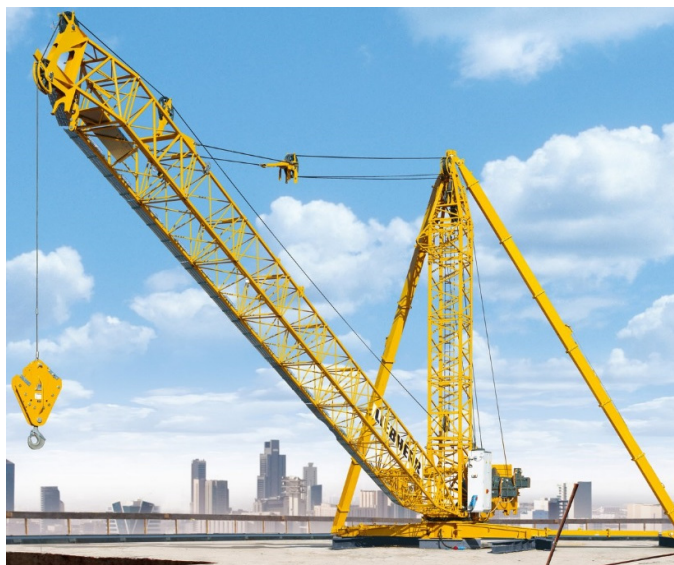
Slika 2.4. Derik kran (slika preuzeta sa internet adrese http://www.eohic.com/construction-equipment/derrick-crane/derrick-crane-35m-3-6-18t.html dana 28.09.2023. god.)
