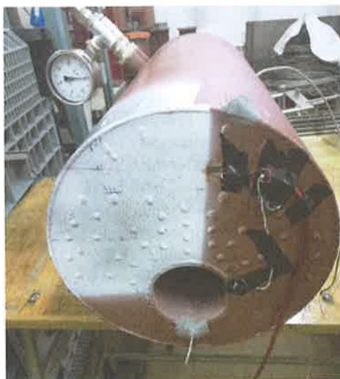
Fig. 5. The strain gauges locations and measuring areas for DIC system
