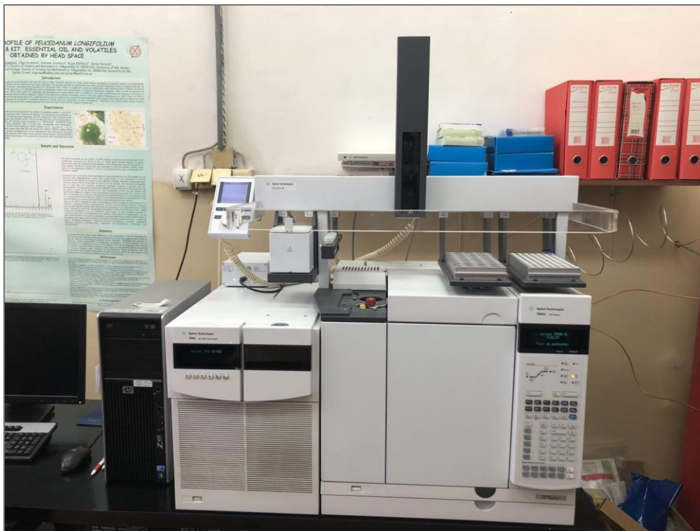
Slika 3.6 7890/7000B GC/MS/MS aparat
