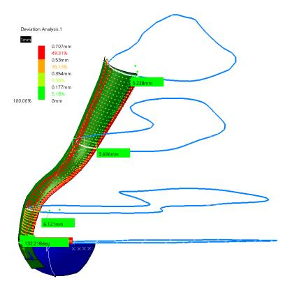
Figure 28 .Deviation analysis between plate contact surface and bone outer surface
