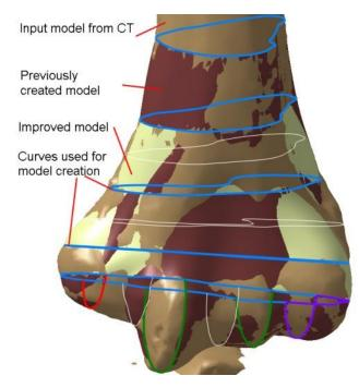
Figure 25.Surface models and spline curves of the distal humerus
