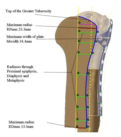
Figure 20.Defined dimensions (parameters) of the humerus bone presented in AP plane
