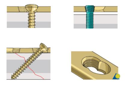
Figure 5. Locking and convetional Screw -Both can be used in Locking compression Plates combination holes [43]
