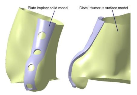
Figure 29 Example of plate implant solid model
