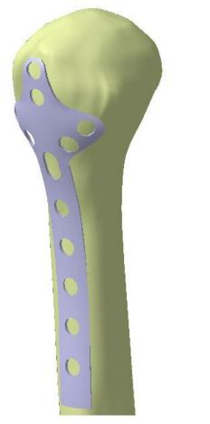
Figure 23. Assembly of the customized plate solid model and surface model of the test humerus
