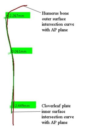
Figure 24.Deviatins in AP Plane between intersections of AP plane and plate surface model, and humerus surface model
