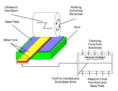
Figure 13. Simplified model of ultrasonic sheet metal 3D Printing[104]
