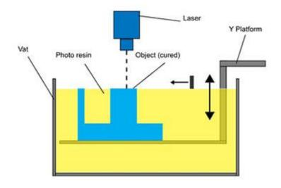
Figure 8. Vat photopolymerisation process[104]
