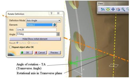
b) TA angle definition Figure 22.Parameters difinition
