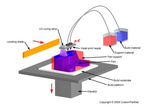
Figure 9. Material Jetting Process [104]
