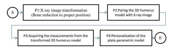
Figure 34 Process for the creation of the personalized plate model for the humerus bone.
