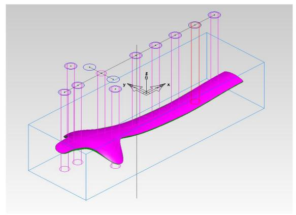
Figure 54. Implant plate model in the CAM software
