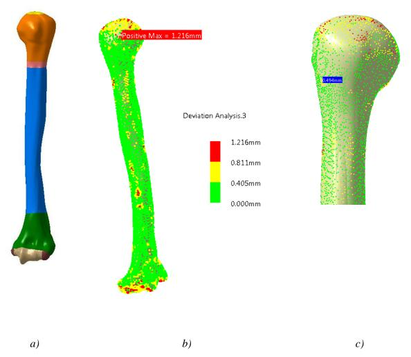
Figure 19. Surface model of the humerus and deviation analysis between created and input model
