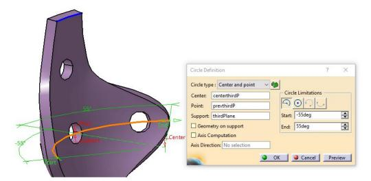
Figure 31. Circle arc definition with Start and End point, and arc angle.
