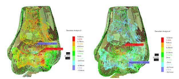
b) Deviation analasys between input polygonal model and previously created surface
