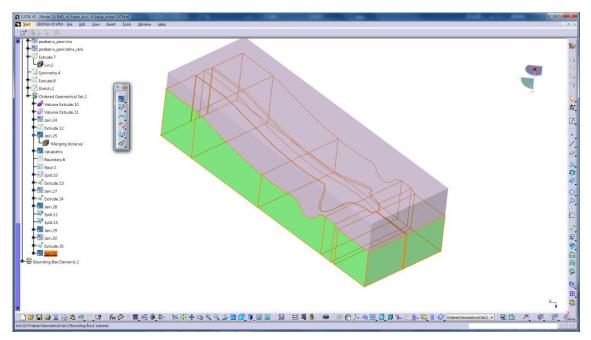
Figure 56. CATIA - CORE and CAVITY design
