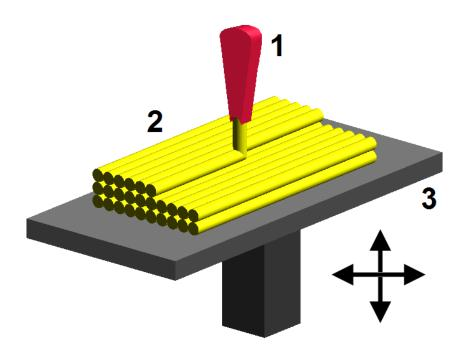
**Figure 11.**Fused deposition modeling(FDM), ,a method of rapid prototyiping: 1 – nozzle ejecting molten material (plastic), 2 – deposited material (modeled part), 3 – controlled movable table. [104]
