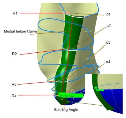
Figure 27. Difined parameters and surface model of the bone-plate contact surface
