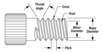
Figure 4.Screw thread parameters<sup>2</sup>.
