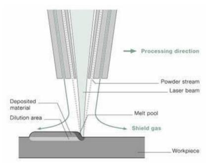
Figure 14. Direct Energy metal powder and laser melting. Image source: Merlin project [104]
